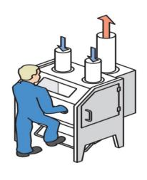
**Diagram 2** Side hood ventilation for an open surface tank
