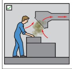
**Diagram 5** Poor design carries contaminants through the breathing zone
