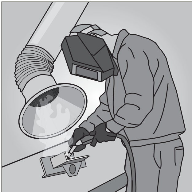
Figure 4: A local exhaust ventilation system with a movable hood is an example of an engineering control.
