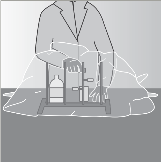
Figure 2: An inflatable glove bag is an example of an isolation control.
