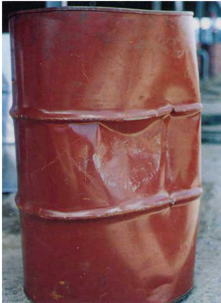
A large dent. NOT ACCEPTABLE The dent is too deep to be blown out satisfactorily. Note the damage to the swedged rolling hoops. These sharp indents are potential leak areas.
