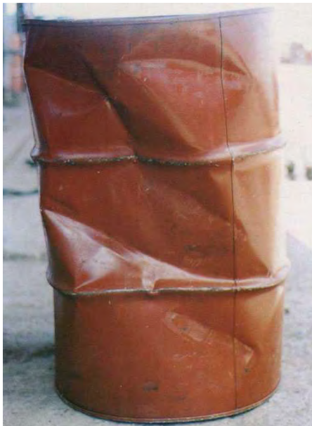
Deep dents. NOT ACCEPTABLE The 5 dents shown in the photo are too deep to be blown out successfully. Note the sharp dents in both swedged rolling hoops, which are potential leak areas.
