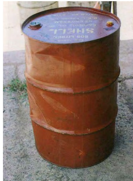
Shallow dents. ACCEPTABLE. Can be blown out sufficiently to make the drum usable.
