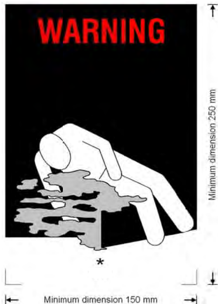
Figure 5.5.2: Asphyxiation warning mark for cargo transport units
