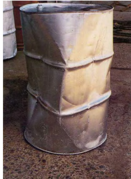
Major body denting. NOT ACCEPTABLE The dents cannot be blown out. Note the damage to the swedged rolling hoops. The sharp indentations will be the site of leaks.
