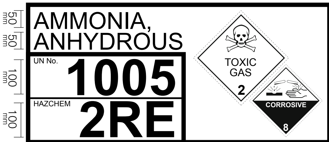
Figure 8: Sample placard for bulk dangerous goods
